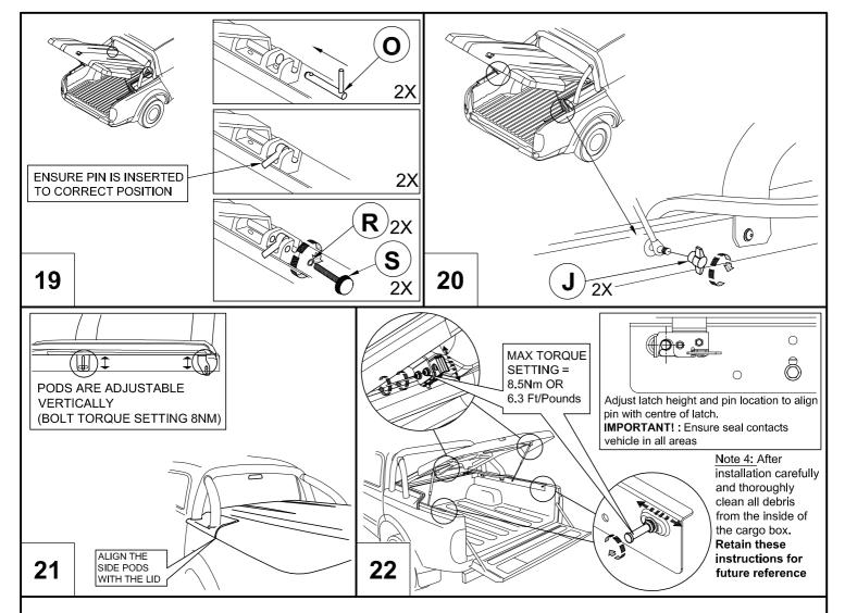
Ensure all bolts are fastened to their stated torque setting once adjustment is complete
